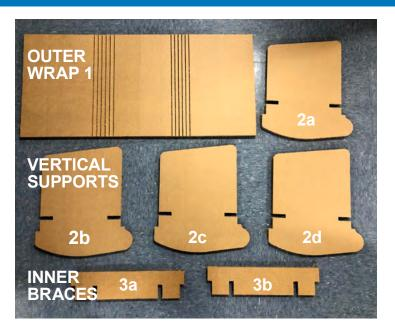
Create Your Own Parts: AAD has precut the parts for this rocking perch project, but our adaptive devices are typically measured and cut by hand. Cardboard is a great material to build with because it can be easily manipulated and cut into any shape you like!
