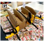
methods to secure multiple glued cardboard pieces is to use drywall screws with a hand drill (**IMAGE F**), or by using adjustable bar clamps as shown in the pictures (**IMAGE G**). You are getting close!
