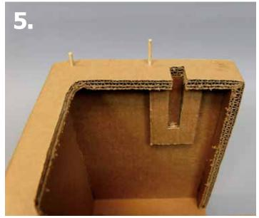
The slotted cardboard pieces are joined to the standing frame with Elmer's glue and dowels. Slots are also carved out of the top of the standing frame to allow access to the slotted cardboard pieces aligned below.
