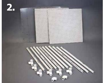
Four walls are created from pegboard, hardboard, and plexiglass. These walls will make up the left, right, rear and top of the rectangular prism. Holes are drilled along the outside perimeter of both the hardboard and the plexiglass to allow for these walls to be mounted with zip-ties. Smaller holes are also drilled in a linear pattern throughout the plexiglass to allow for items to be strung down through from above once it is mounted.
