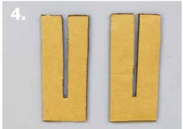
Separate pieces are cut out for the slot mechanism that will be used to hold the child upright within the standing frame.
