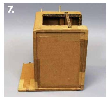
Heavyweight paper applied with Elmer's glue is used to cover the exposed corrugate edges of the device, holes where dowels were driven through, and any other torn or punctured areas of the cardboard.
