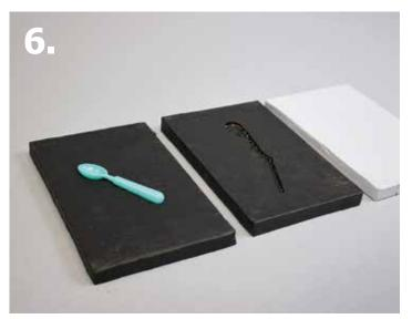
An item that will represent a specific activity is chosen to be placed on the tactile cue. The silhouette of that specific item is drawn onto the center of the cue. That pattern is then carved out of two layers of the cardboard cue. The cue is primed, painted and polyurethaned, and the chosen item is hot glued into its corresponding hole.
