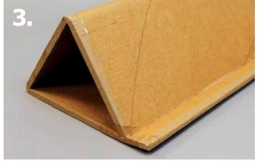
Heavyweight paper applied with Elmer's glue is used to cover the exposed corrugate edges of the device and any other torn or punctured areas of the cardboard.
