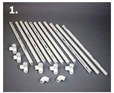
One inch PVC tubing is measured and cut to length to make a custom sized rectangular prism that will fit around the child. Three out of the eleven PVC tube segments are cut longer to create a wider shaped rectangular prism instead of a perfect cube where all the sides are the same length. Six three-way elbow fittings, and two two-way elbow fittings will be used to join all of the straight PVC tubing segments together.
