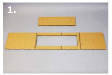
Measurements are taken of the product's end-user to create an ergonomically correct pattern from. The pattern is then drawn onto a sheet of tri-wall cardboard, and cut out using either a utility knife, jig saw, or band saw. Lines are marked on the template to show where bends, scores, and grooves will be made.
